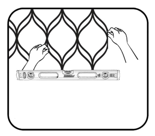
3. Start the application aligning the panel on the top left corner of the wall. Make sure it is leveled and will work with the panel you will apply on the right and bottom. Now you are ready to apply.
