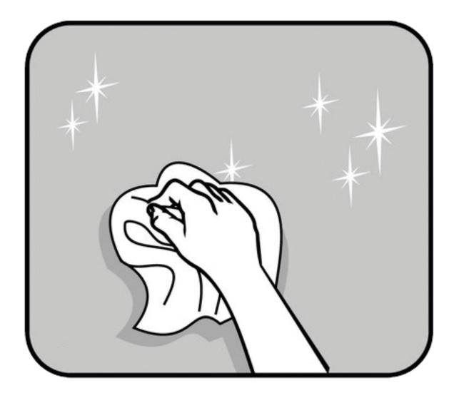
1. Clean the surface, make sure the surface is free of dust, dirt and moisture. Let it dry.
