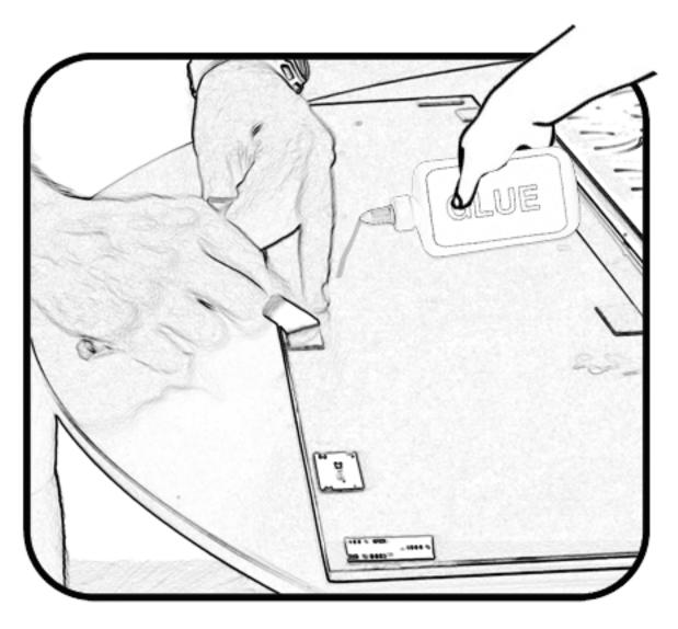
2. Apply the Double Sided Adhesive Tape or apply Liquid Nail Adhesive in the back of each panel.
