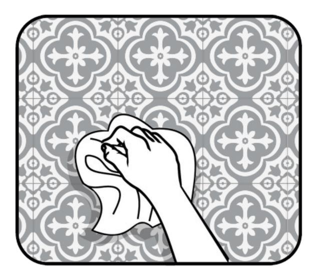
3. Adjust as needed then press firmly with a smooth cloth from top to bottom, carefully pushing out any air bubbles.
