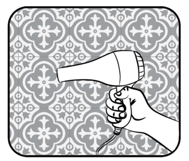
4. With a hair dryer apply some heat to the tile stickers to activate the glue and seal it. Make sure you do this process on the edges.
